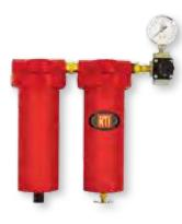
**STEALTH 6060B** .5in (13mm) inlet dual-stage filter system with .375in (10mm) final regulator and first stage auto drain. It uses activated carbon to remove water, dirt, oil, oil vapor and includes two BK-1 mounting brackets.
