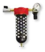
**MD4** 1.0 micron filter with 4 layer filtration, .5in (13mm) inlet, ball valve, and manual drain. Provides oil and humidity free air, has .25in (6mm) regulator with gauge. Includes mounting bracket. Perfect for DIY or small volume shops.
