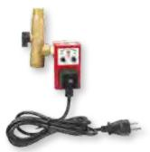
**ED-2-4** Electronic timer drain with indicator lights. Automatically drains water from tank and features a solid brass ball valve with stainless strainer to protect the valve. Manual override comes standard, fits .25in (6mm) or .5in (13mm) NPT.
