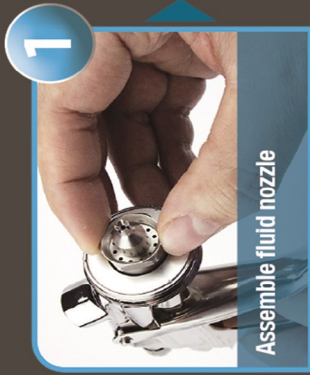
Tighten up the fluid nozzle with spanner wrench*
