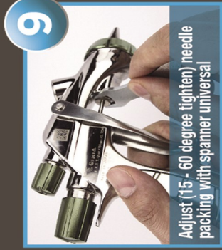
Check the trigger and needle travel smoothly
